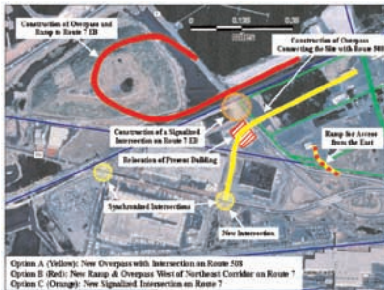
Figure 4.14 Transportation Improvement Options at Koppers Coke Site
