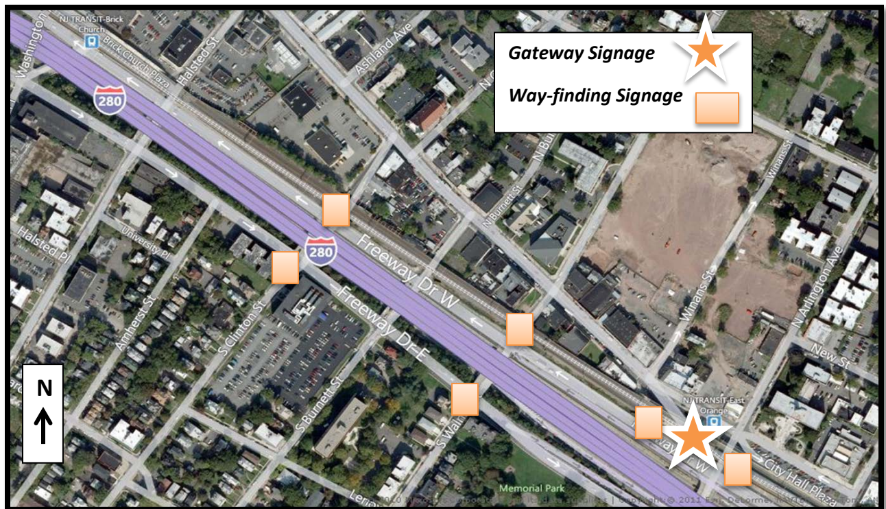
Figure 6: Recommended Location of Signage along Freeway Drive
