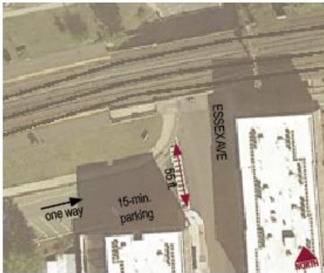
The one-way lane exiting the station area near the 15-minute parking has a large turning radius on the northwest corner and measures 55-feet wide at the pedestrian crossing point.
