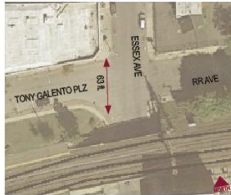
The southwest corner has a large radius and the pedestrian crossing distance is 63 feet. Longer crossings expose pedestrians to more vehicular conflicts and a wider radius facilitates faster turning movements.
