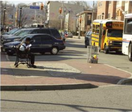
Though the current reverse angle parking configuration allows for an easy parking space entrance, it requires that vehicles exiting the parking space back up into a live travel lane.
