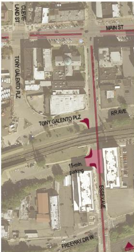
The one-way lane exiting the station area near the 15-minute parking has a large turning radius on the northwest corner and measures 55-feet wide at the pedestrian crossing point.
