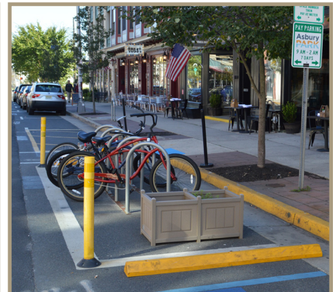
Figure 27. Yellow plastic bollard, parking stop, plastic planter, bike parking. Asbury Park, New Jersey.
