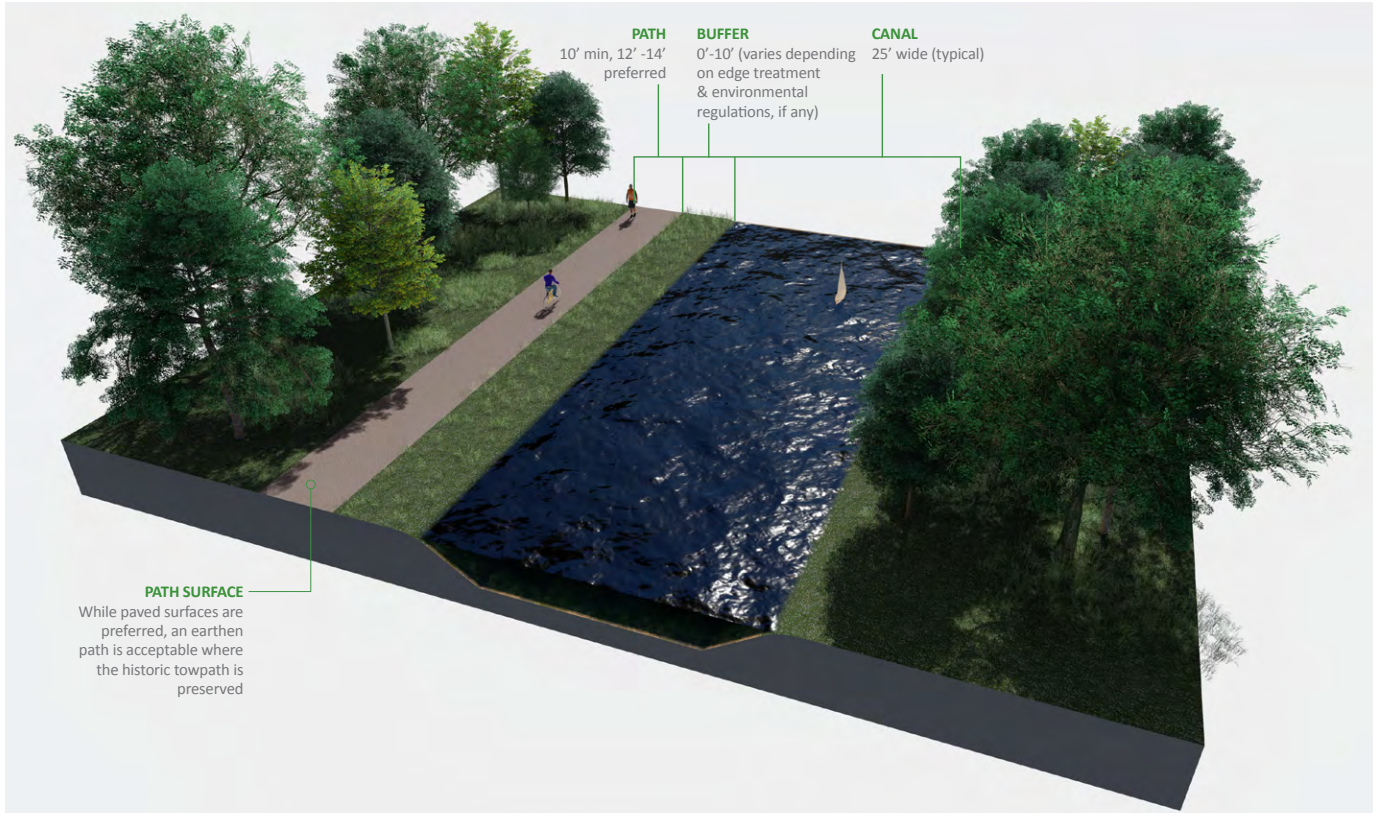
Figure 3.1. Canal-Side Shared Use Path Cross Section
