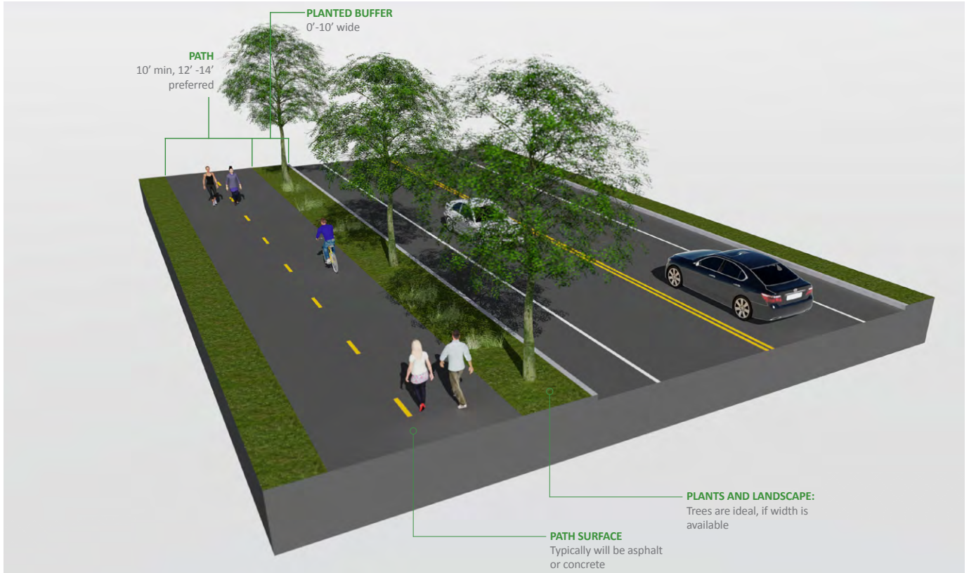
Figure 3.3. Road-Side Shared Use Path Cross Section
