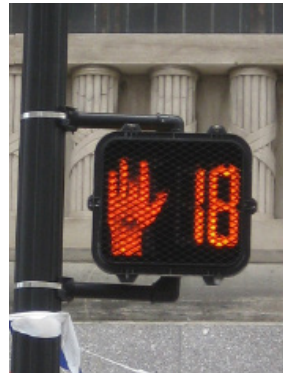
A pedestrian signal on Broad Street indicates when pedestrians have the right-of-way and how much time they have left to cross.
