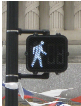
A pedestrian signal on Broad Street indicates when pedestrians have the right-of-way and how much time they have left to cross.
