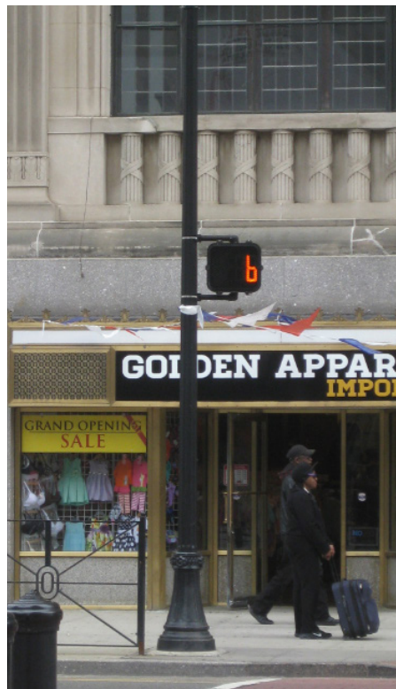
A pedestrian signal on Broad Street indicates when pedestrians have the right-of-way and how much time they have left to cross.
