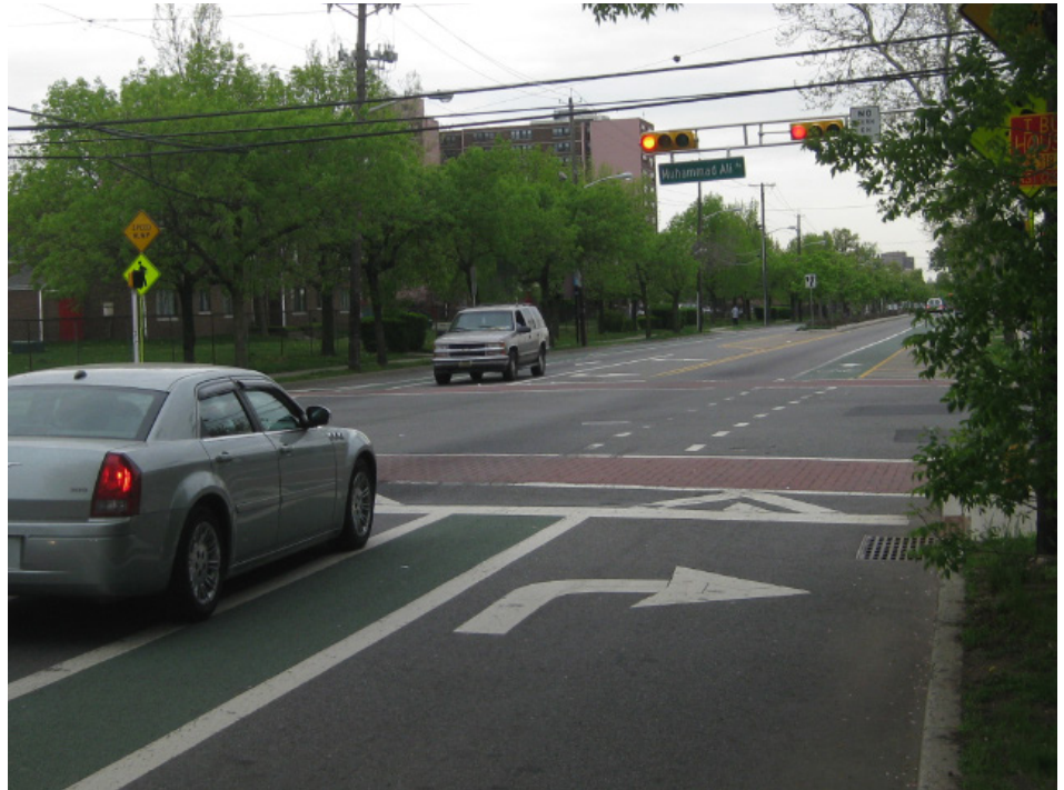
A raised intersection also acts as speed table at Irvine Turner Boulevard and Muhammad Ali Avenue, providing better visibility of pedestrians and calming traffic.
