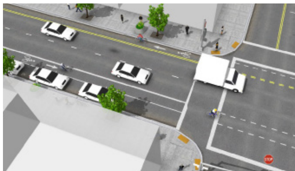
Contra-flow bike lane schematic from the NACTO Urban Bikeway Design Guide.
