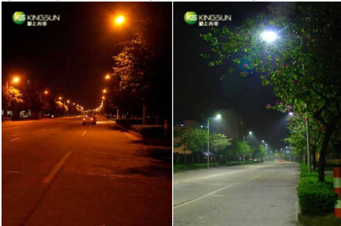
Figure 3: Comparison of a street lit by HPS (left) versus LED (right)
