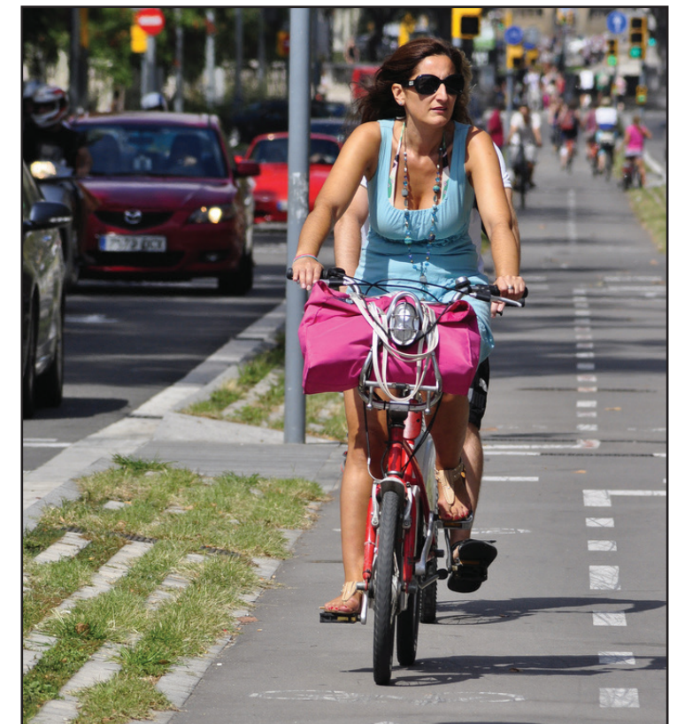
Grass Pavers Form the Edge between the Roadway and Bikeway, Barcelona, Spain
