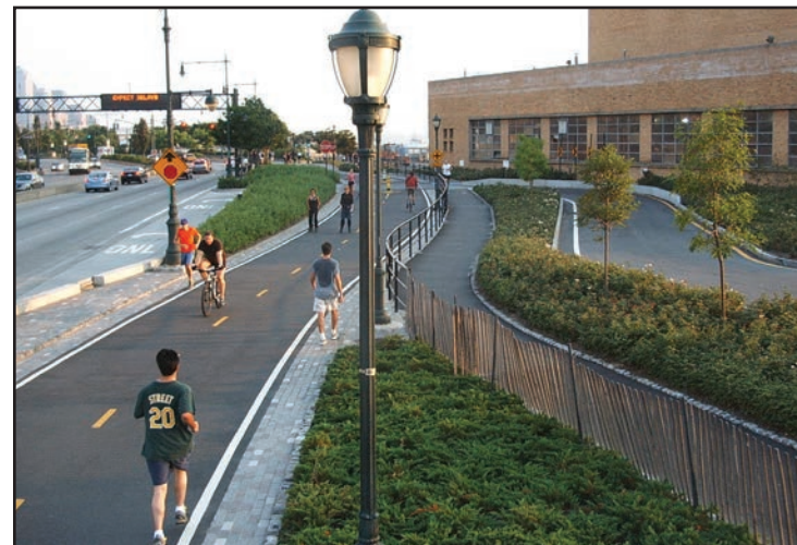
Off-street Multi-use Pathway with Planted and/or Fenced Separation Between Bicyclists and Pedestrians Along the West Side Highway in Manhattan, New York
