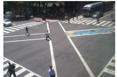
Intersection with exclusive pedestrian phase
