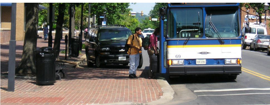
Bus bulbs provide a convenient boarding area for bus riders
