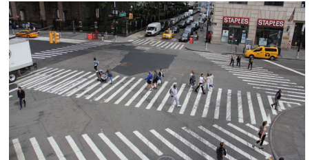
Intersection with exclusive pedestrian phase
