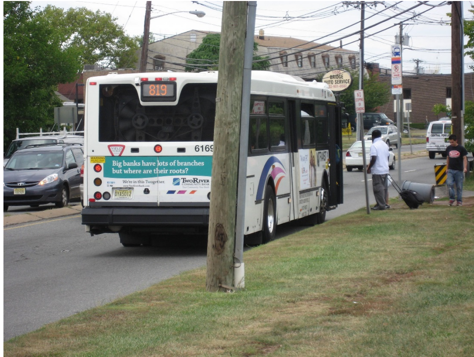
Bus stop on Route 529 between Metlars Ln and Hadley Rd, serving Middlesex Mall and Hadley Center; no shelter and no sidewalk; worn pedestrian paths are present (August 21, 2014; IMG_2764)
