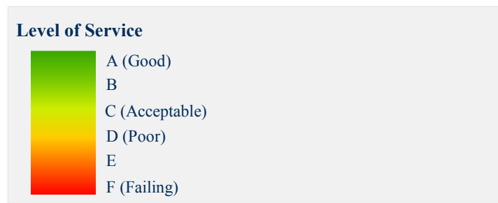
Figure 24 - Level of Service (LOS)
