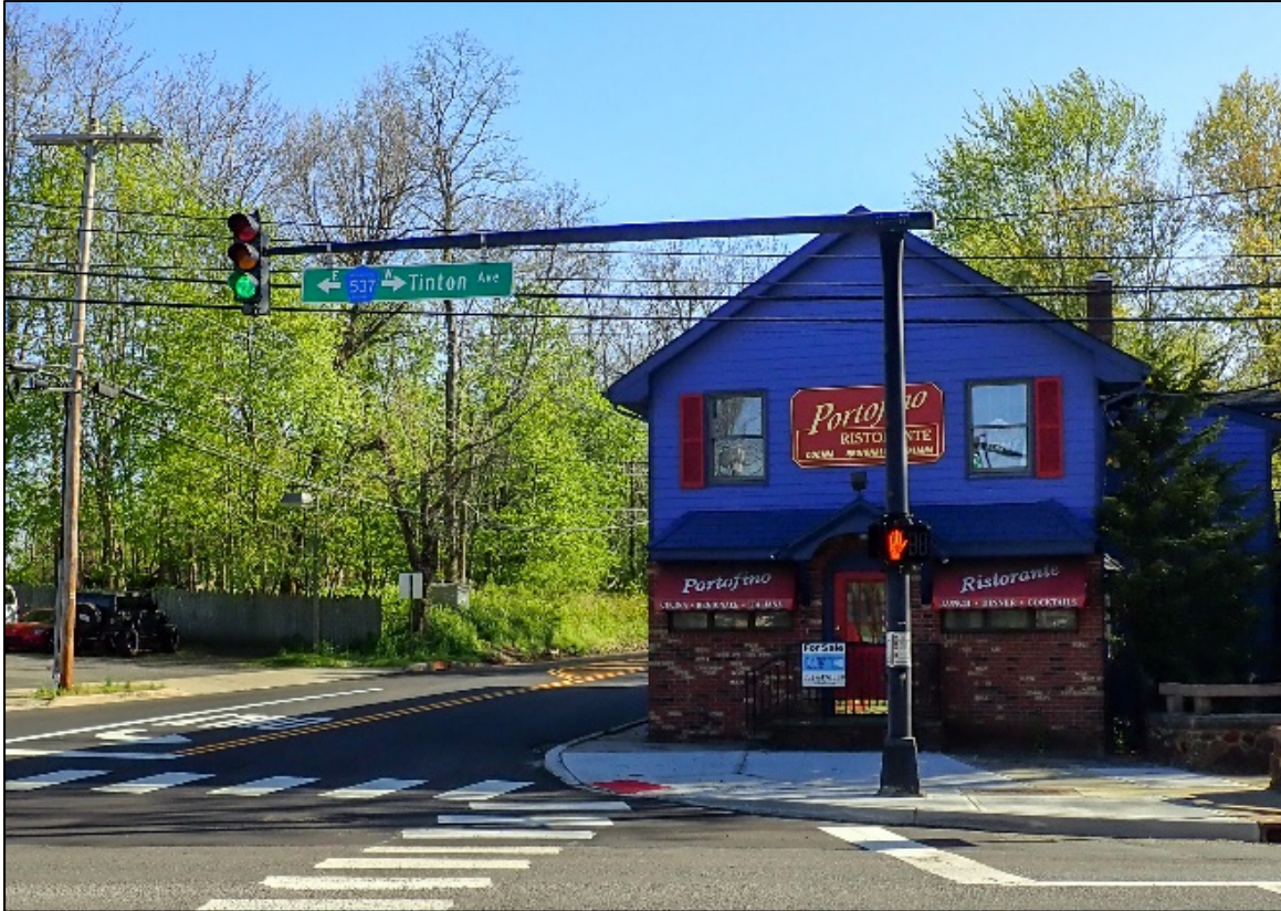
Figure 31 - Context Sensitive Signals in a Historic District, Tinton Falls, NJ
