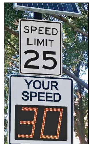
Figure 24 - Example VMS Speed Sign
