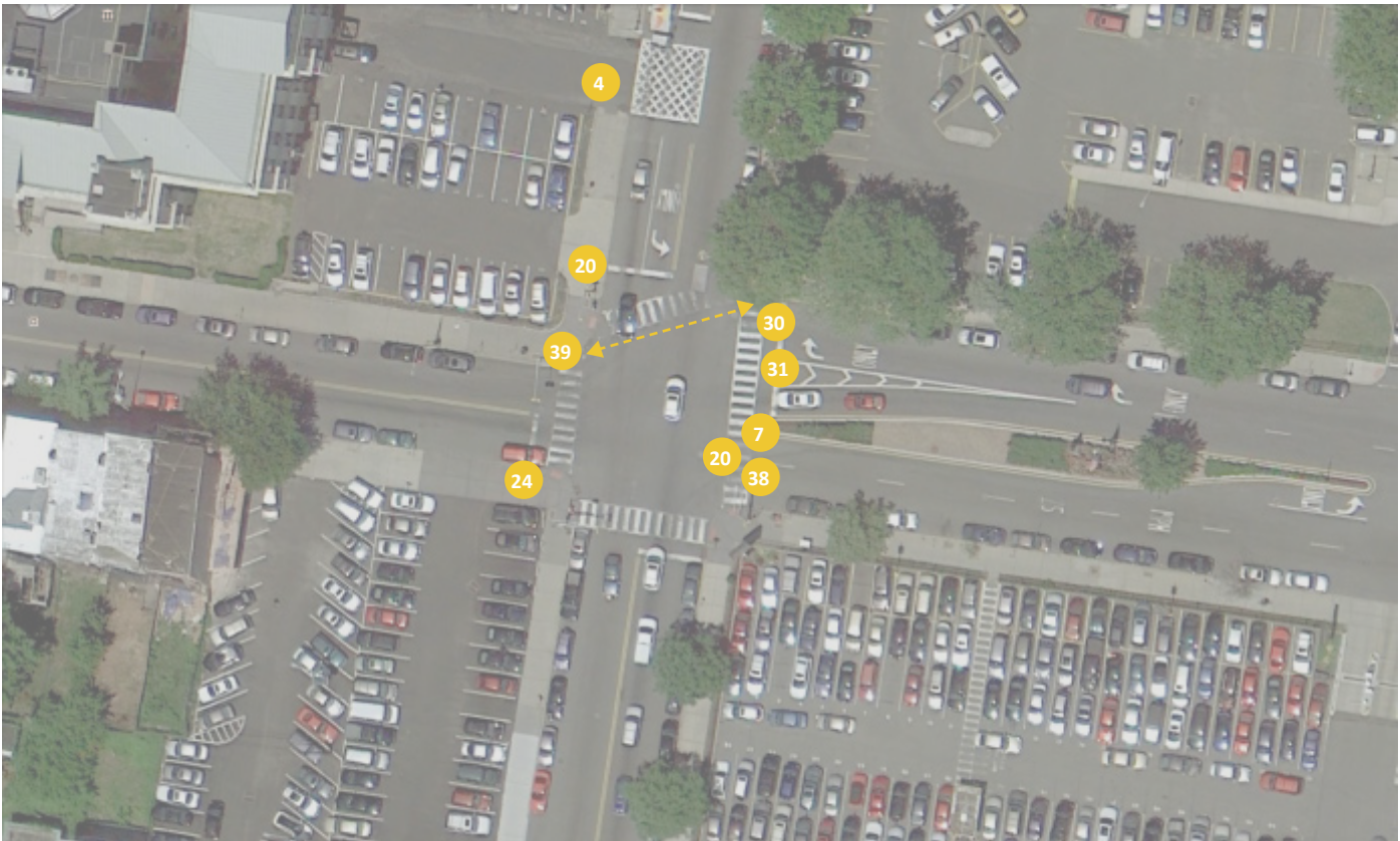
Westbound bicycle lane approach for straight-through movement conflicts with right-turning vehicles
