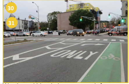
Westbound bicycle lane approach for straight-through movement conflicts with right-turning vehicles
