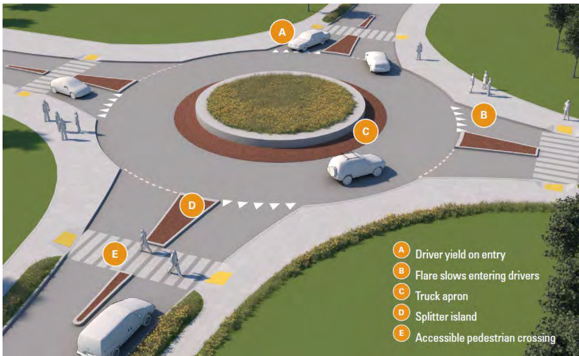
Figure 19 – Roundabout Example (Source: CSDG)
