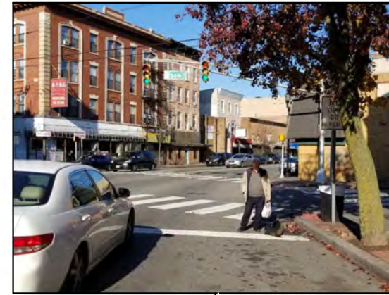
Many signs are partially obstructed by roadside objects along Bergen Avenue.
