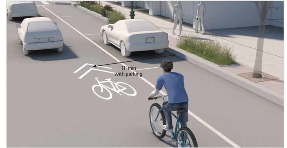
Typical Sharrow design and pavement markings
