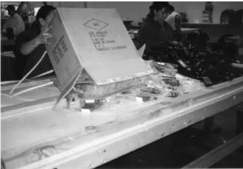
Photos A-3 through A-5. Retail Distribution Center System - Value-added services provided commence with the unpacking of a shipment of adapters that will then be kitted together with seven different components shipped from other countries. An assembly line process facilitates the packaging operation in which the items are packed in custom designed heat sealed plastic packaging along with a cardboard backing sheet. Finished packages (shown below on far right of photo) are then shipped directly to retail outlets.
