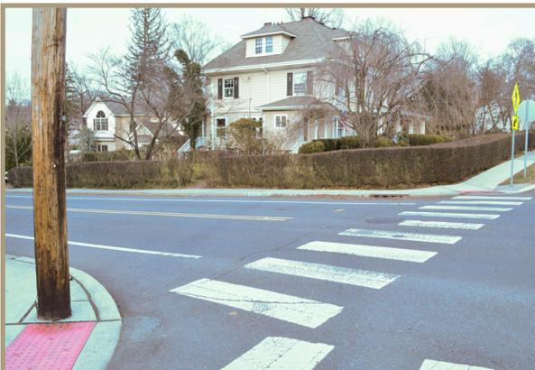
Figure 37. High visibility crosswalks, ADA compliant ramps, and pedestrian signage at Mt. Airy Road.
