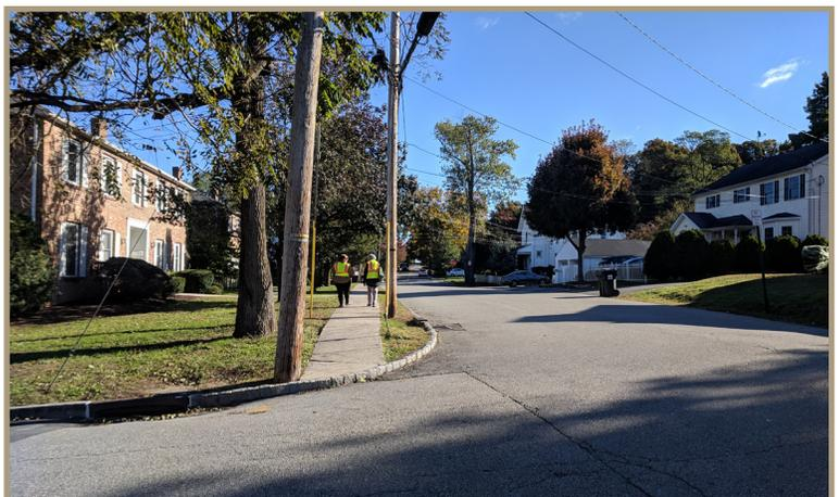
Figure 18. Sidewalk lacking wheelchair accessible ramp, and no painted crosswalks in any direction.
