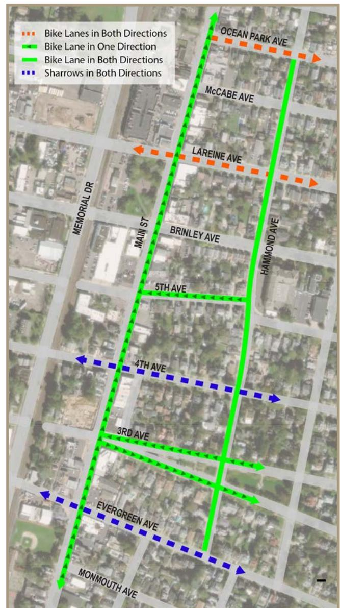
Figure 55. Proposed bicycle network along Main Street and connecting roadways in Bradley Beach.
