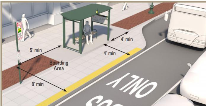
Figure 62. Bus bulb design standards. (Photo Credits: NACTO)
