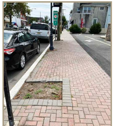
Figure 18. Tree wells on a 9-foot sidewalk north of Fourth Avenue on Main Street.
