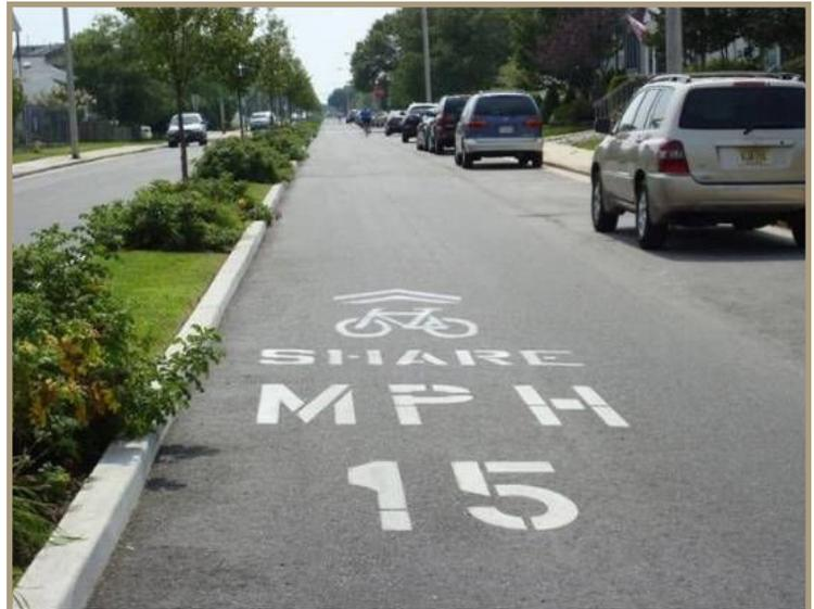
Figure 49. Pavement markings in Ocean City, New Jersey.
