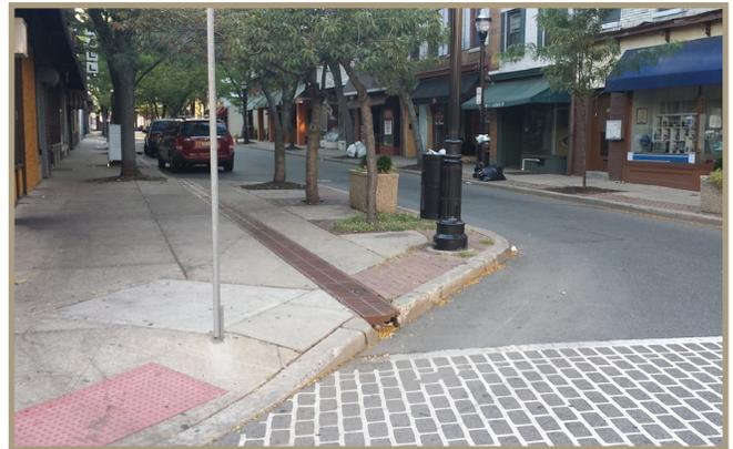
Figure 25. Example of a covered gutter in Rahway, NJ.
