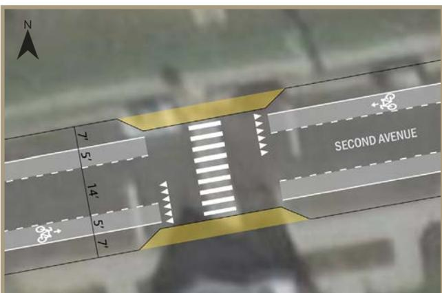
Figure 60. The mid-block crossing in front of St. Anne's Convent with proposed Bicycle Boulevard improvements.
