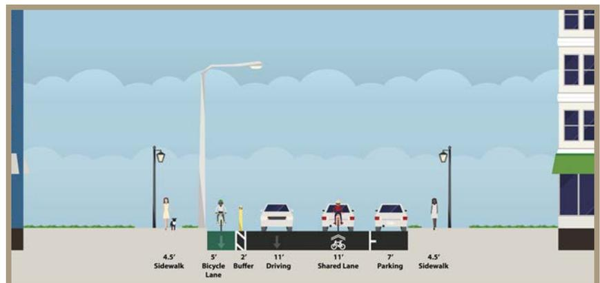
Figure 71. Beech Street with an uphill buffered bicycle lane, shared downhill lane, and added pedestrian lighting.
