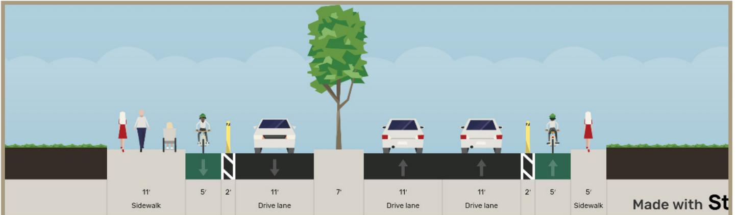
Figure 67. Prospect Avenue with a median and buffered bicycle lanes, looking south.
