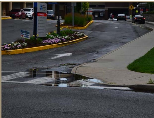
Figure 24. Poor drainage by a hospital entrance.
