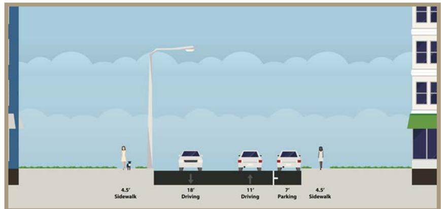
Figure 70. Current Allocation of space on Beech Street, looking east (downhill).
