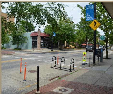
Figure 28. Orange plastic bollard, stop for pedestrian signs, bike parking. Collingswood, New Jersey.
