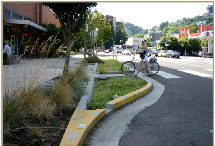
Figure 12. Green infrastructure used to narrow the roadway and provide a shorter crossing distance for pedestrians.
