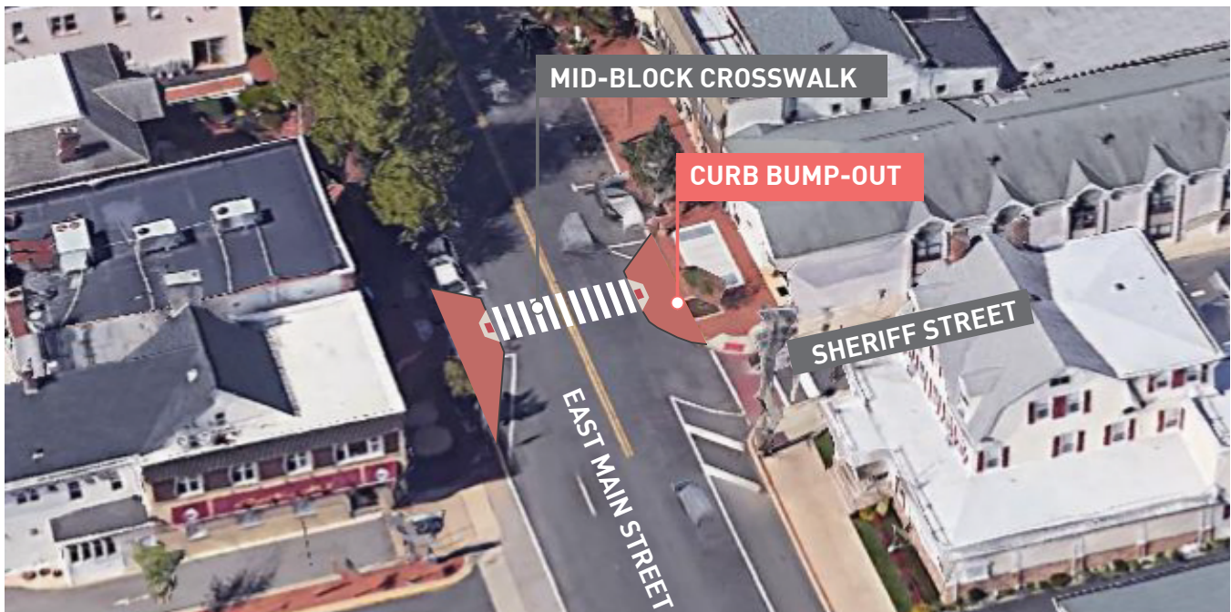
Figure 30: Mid-Block Crossing Design
