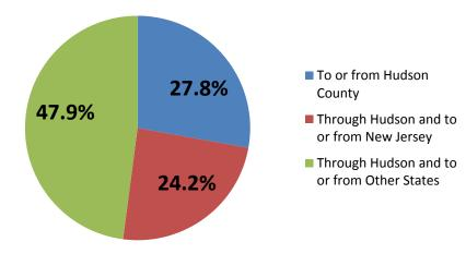
Nearly 48% of trucks traveling on the selected highways in Hudson County were passing through the County on their way between origins or destinations outside the State of New Jersey. About 28% were traveling to or from a point in Hudson County. Just over 24% of trucks on the selected highways were traveling through Hudson on their way to or from locations within the State, but outside Hudson County.
