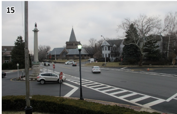
The unsignalized intersection of Park Avenue with Chestnut Street, W. Passaic Avenue, Lincoln Avenue, and E. Passaic Avenue is confusing for motor vehicles, bicyclists, and pedestrians. It features 7 crosswalk legs, the longest of which (shown) is about 160'. (Rutherford_180221_081117.JPG, Rutherford_180221_081212.JPG)
