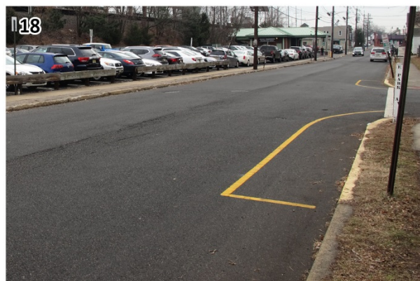
18 Many intersections in the study area were observed to include "daylighting" measures such as what is pictured here, at Pearl Street. (Woodbridge_180122_083619.JPG)
