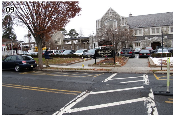
The Curb ramp at Kings Road and Maple Avenue does not align with the curb ramp where pedestrians should cross the parking lot. (Madison_121217_104006.JPG)
