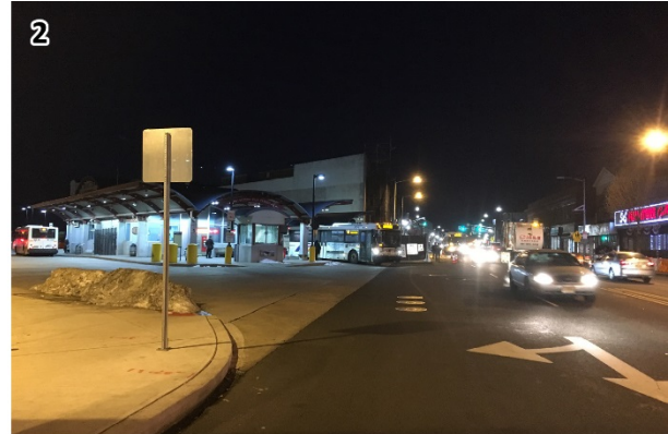
The bus terminal driveway is an elongated pedestrian crossing, but without crosswalk markings or adequate lighting for the middle of the driveway.
