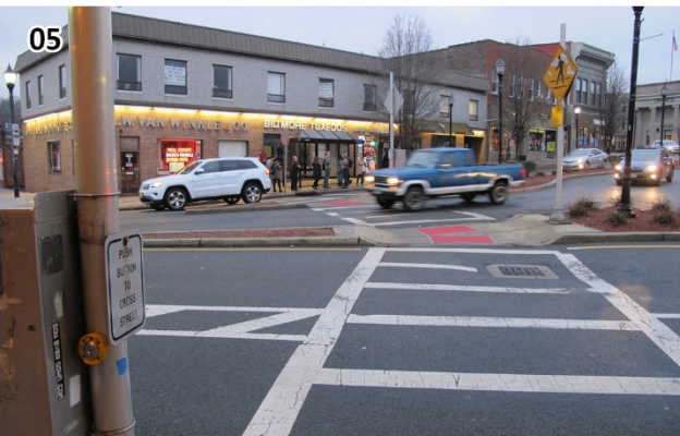
Pedestrian Crossing signs at the station along Erie Avenue include actuation devices but lack blinking signals. (Rutherford_180221_063646.JPG, Rutherford_180221_063720.JPG, Rutherford_180221_064215.JPG)
