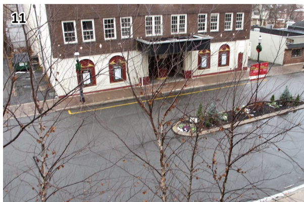
Small planted median on Lincoln Place leaves a wide travel lane, which can be driven as a straight path through the intersection, rather than deflected. (Madison_121217_110824.JPG)
