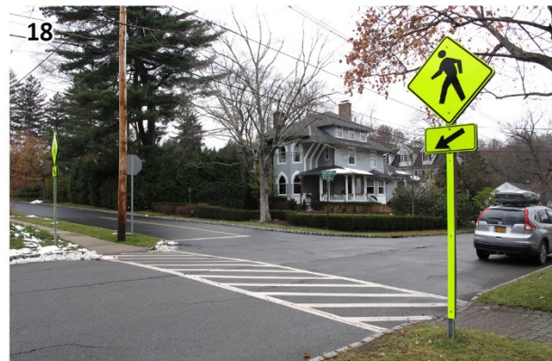
Pedestrian crossing signs assemblies (MUTCD W11-2 + W16-7P) were used throughout the borough, as seen here at Crescent Road and Hillside Avenue. (Madison_121217_142551.JPG)
