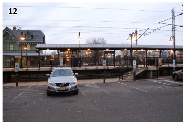
Lot 2 includes (5) ADA parking spaces with an accessible route to a ramp leading to the station platform. The ramp is \pm 200' from the parking. (RedBank_180201_072434.JPG)
