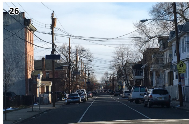
Wide parking lanes visually narrow the moving lanes, effectively slowing much of the through traffic.
