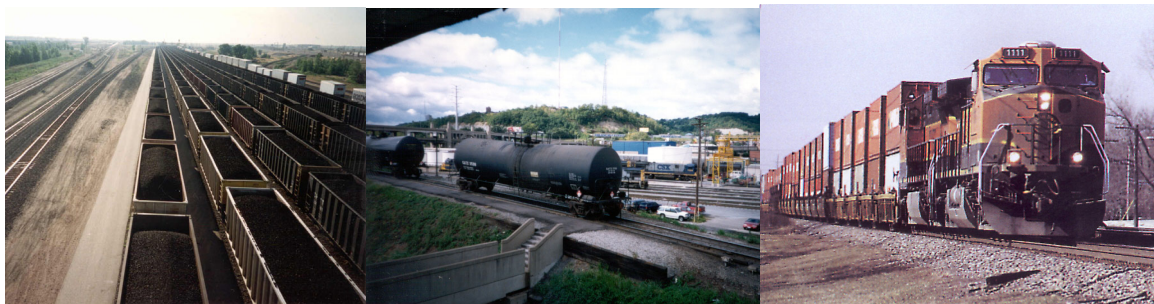
Figure 21. Examples of Unit, Carload, and Intermodal Trains
