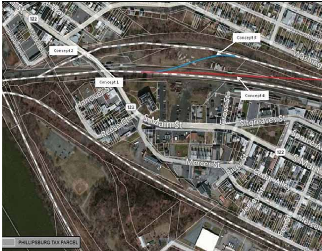
Figure V.2 - Alternative Improvement Concepts to Achieve Plate "F" Clearance at the South Main Street Bridge
