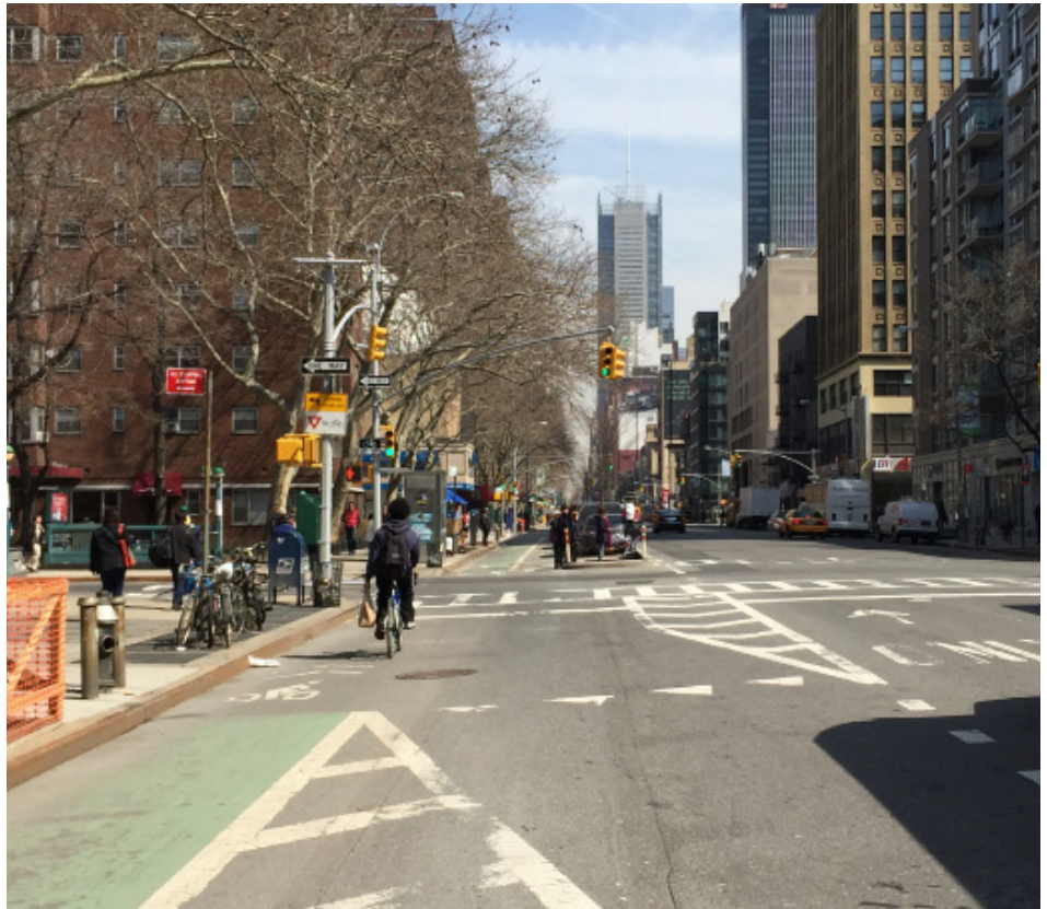
A mixing zone on 8th Avenue in New York City.
