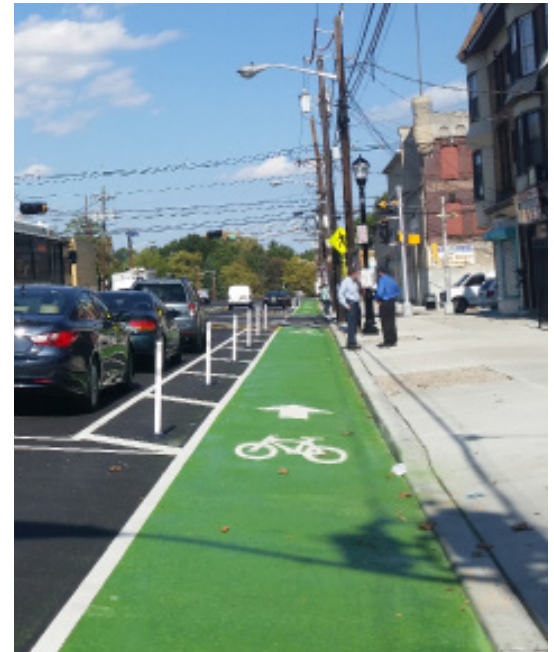
The protected bicycle lane on Mt. Prospect Avenue uses a painted buffer with plastic flexi-posts to separate the bicycle lane from the parking and travel lanes.
