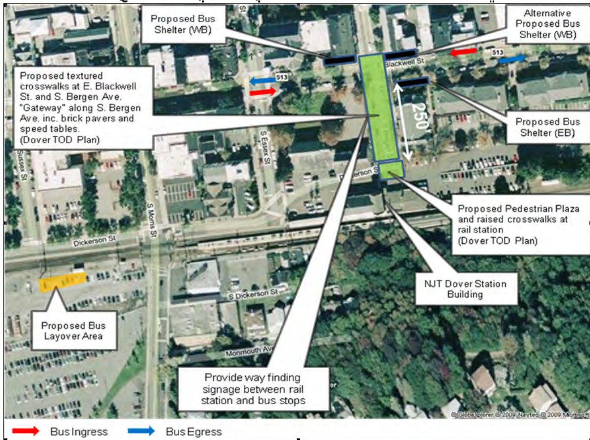
Figure 5-5: Proposed Improvements to Dover Railroad Station
