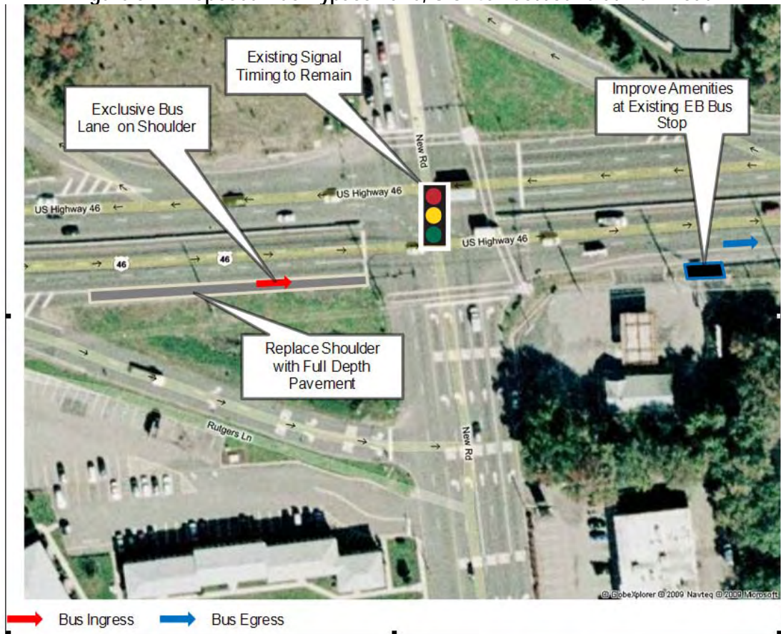
Figure 5-1: Proposed Bus Bypass Lane, U.S. 46 Eastbound at New Road
