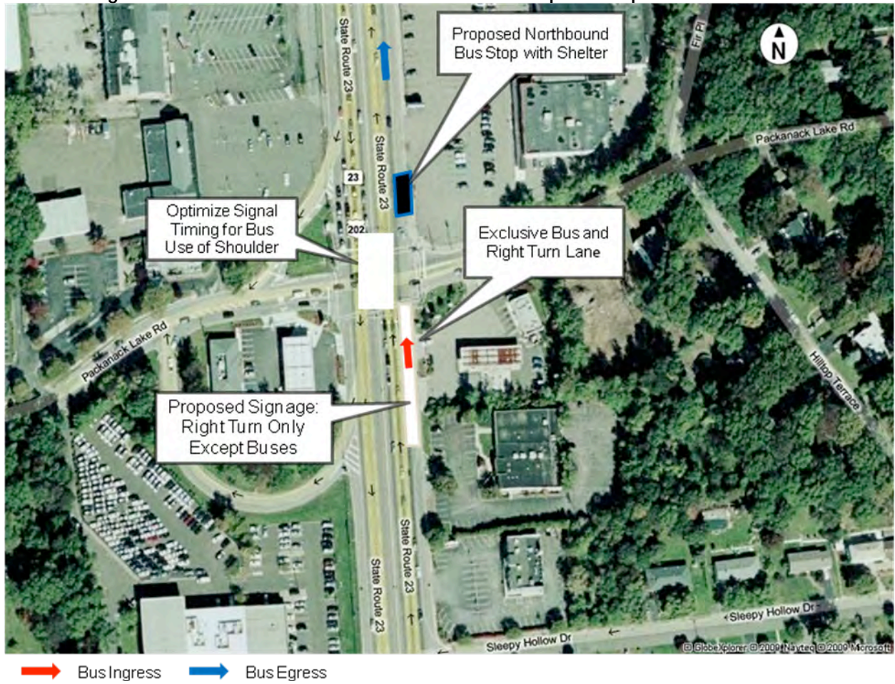
Figure G-4: N.J. 23 and Packanack Lake Road – Proposed Improvements
