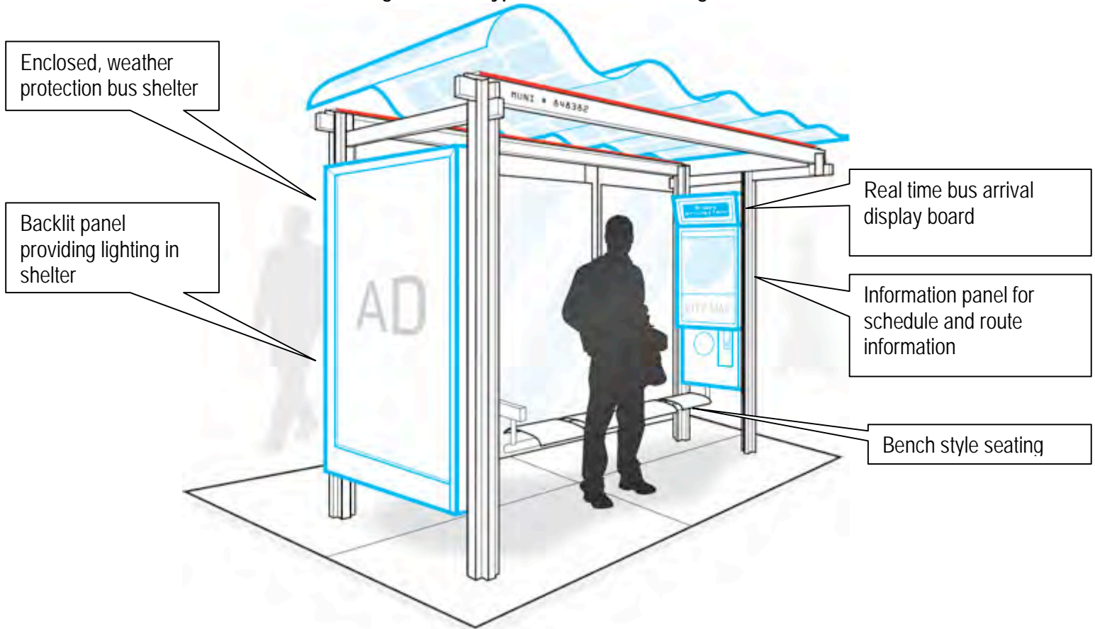
Figure G-15: Typical Bus Shelter Design
