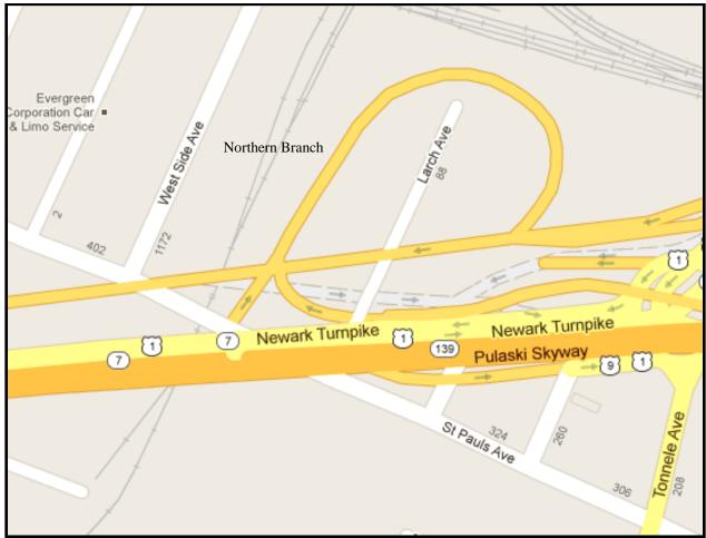
Currently, some CSX traffic from the north diverts at CP Croxton to the National Docks Branch. Due to a trackage constraint entering Greenville yard from the National Docks that negates a progressive move, CSX is evaluating a new route utilizing a to-be-constructed 'Waverly Loop" that would reroute Greenville-bound traffic to run via the P&H Branch.
