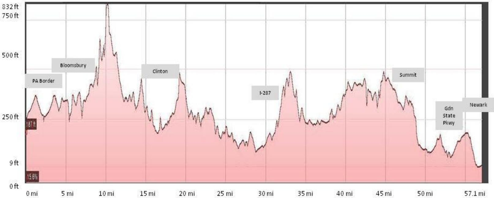
During construction, the peaks and valleys noted in the figure above will need to be leveled over the length of the rail to allow for efficient and cost effective rail operations. Although not completely identified, it is estimated that the mass haul movement, or earthworks, for this project could exceed 50 percent of the overall cost of development, or about \$540 million dollars.
