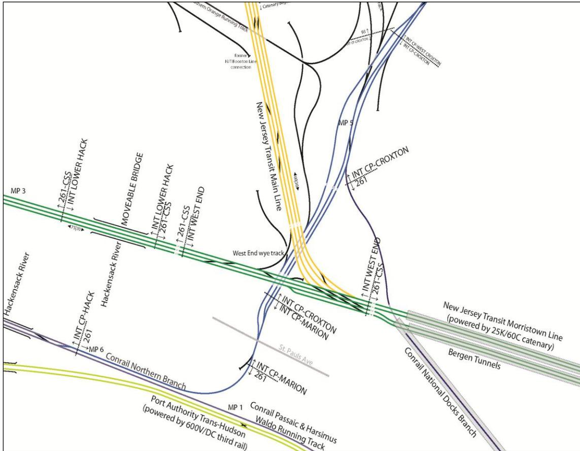
P&H is double-tracked between Waverly Yard and CP-Hack but, effectively, only a single track exists for through freight movements between CP Kearny and CP Hack. The moveable bridge is a two-track structure but, for all intents and purposes, the south track is dedicated to the South Kearny intermodal terminal facility when they need to switch trains in and out of the facility.
