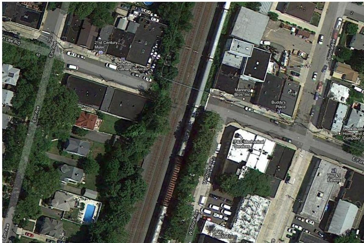
This crossing was not listed as a previously studied crossing but was encountered during the mapping of the triple tracked portion of the River Line through Bogota. While not listed as a problem crossing location in the previous grade crossing study, due to the increased volume of rail traffic and the unusual crossing configuration located close to a key Interlocking, the HDR Team believes it was prudent to bring our observations to the NJTPA’s attention.
