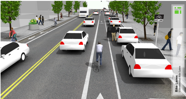
Example of Bicycle Lanes Next to On-Street Parking and a Curb
