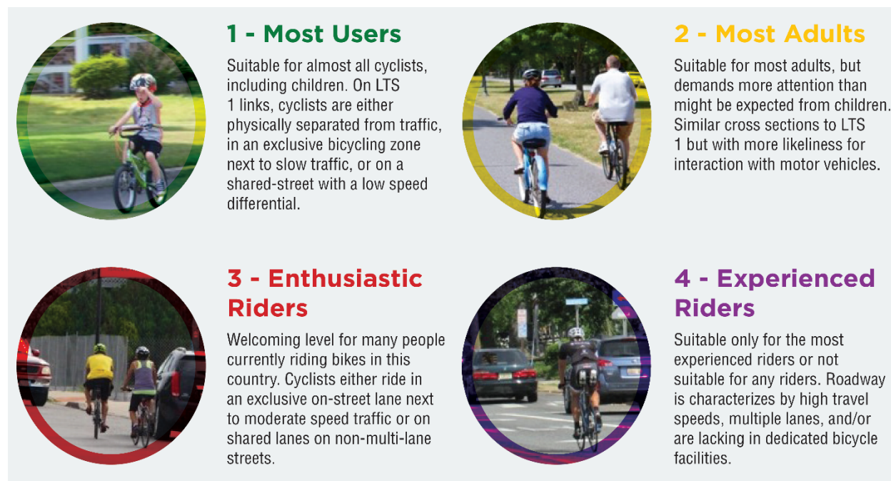
Figure 4: The Four Types of Bicyclists by Level-of-Traffic-Stress (LTS)
