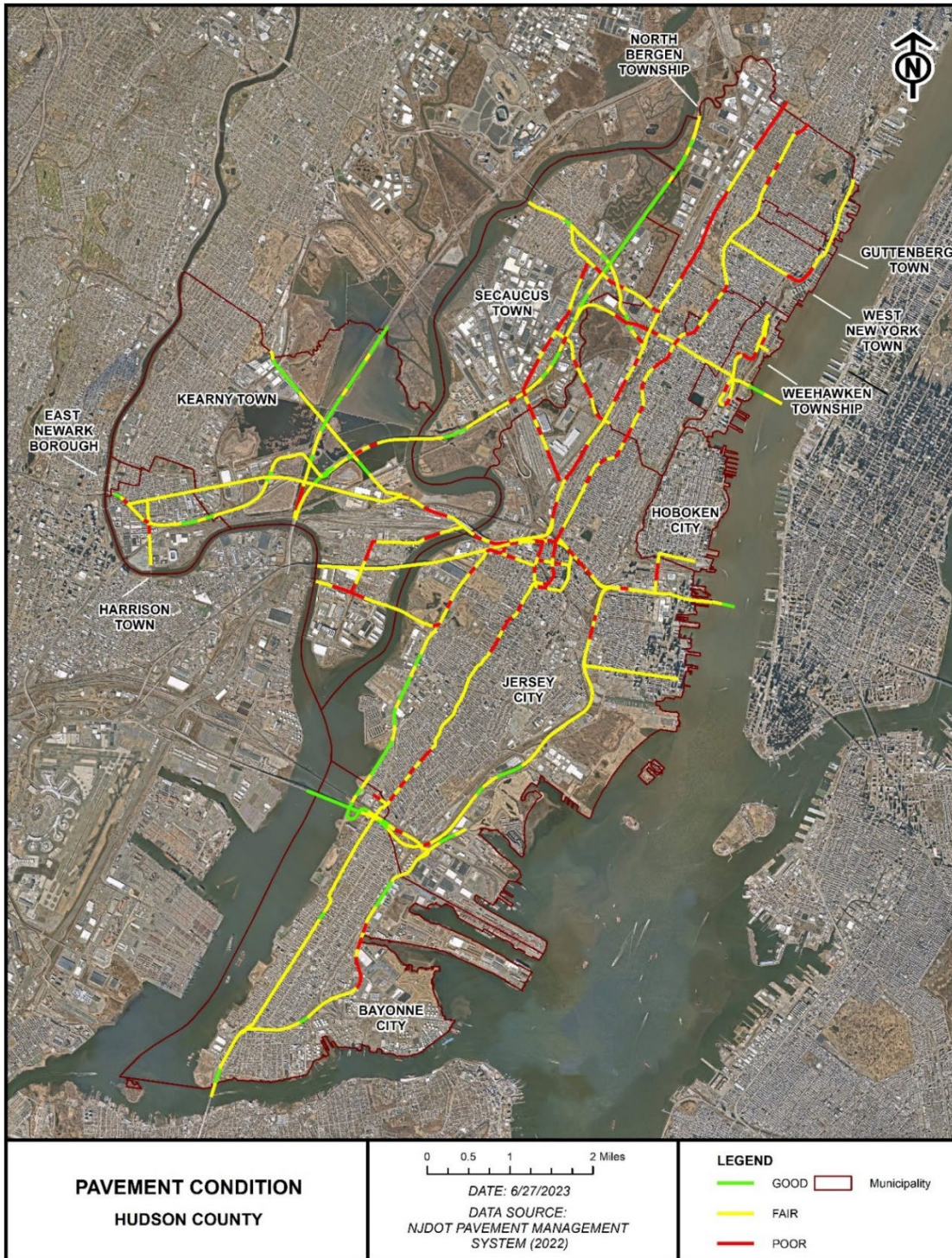
Figure 5: Pavement Condition (Source: NJDOT Pavement Management System)
