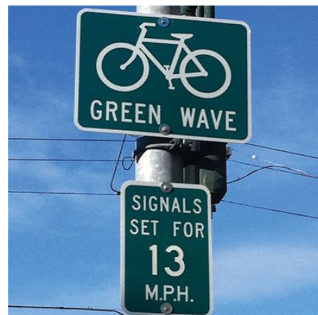
Advisory signage that tells drivers what speed the signals are set for can encourage drivers to maintain that speed. Source: ITE/Nelson Nvaard
