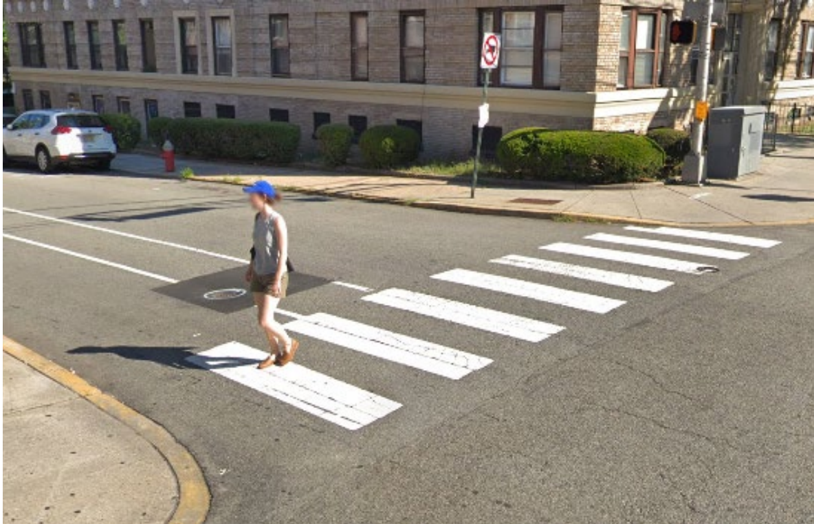
A high-visibility crosswalk at Glenwood Avenue and Kennedy Boulevard. Source: Google Street View
