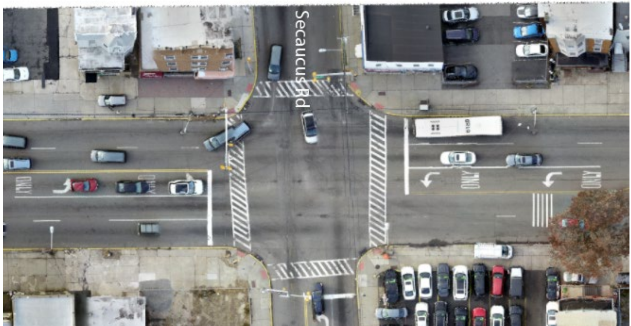
Aerial of Secaucus Road and Kennedy Boulevard, where dedicated left-turn lanes were installed Source: Hudson County
