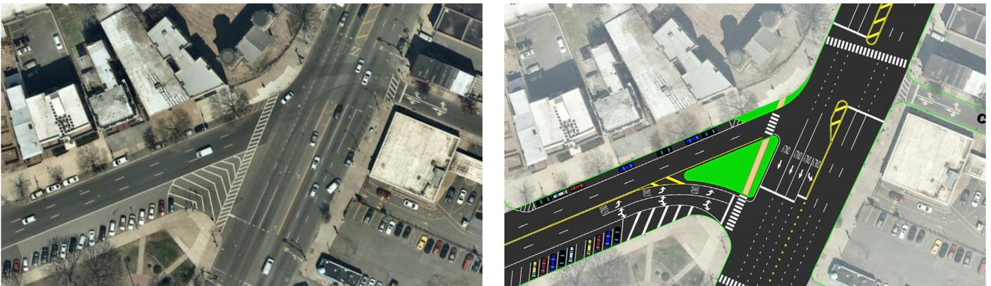
**Figure 34: Existing and Recommended alignment of Intersection**
