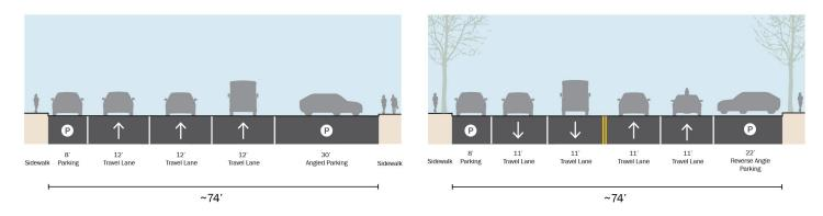
Figure 33: Existing and Recommended Cross Section of Lincoln Park between Clinton Avenue and Broad Street (looking north)
