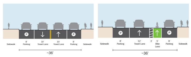
Figure 38: Existing and Recommended Cross Section of Pacific Street (looking north)
