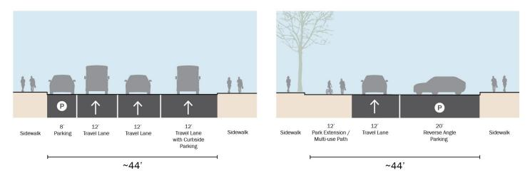
Figure 25: Existing and Recommended Cross Section of Park Place (looking north)
