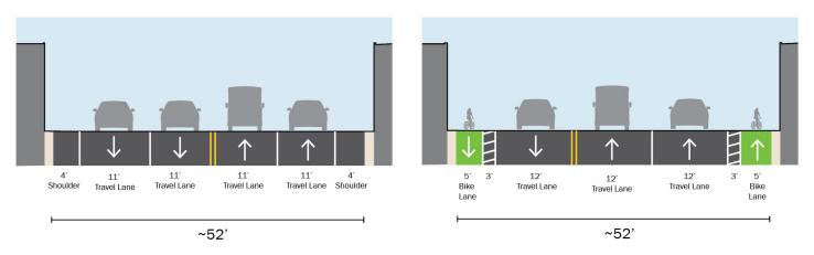
Figure 20: Existing and Recommended Cross Section of Raymond Boulevard (looking west)
