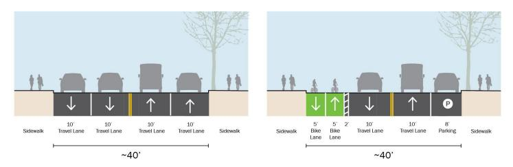
Figure 30: Alternative 1: Existing and Potential Cross Section of Central Avenue (looking west)
