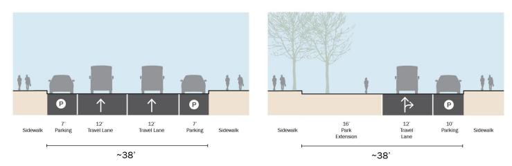
Figure 18: Existing and Recommended Cross Section of Sussex Avenue (looking west)
