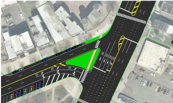
Figure 34: Existing and Recommended alignment of Intersection
