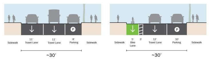
Figure 19: Existing and Recommended Cross Section of University Avenue (looking south)
