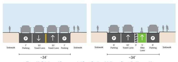
Figure 39: Existing and Recommended Cross Section of Jefferson Street (looking south)
