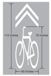
*Figure 23: Dimensions of a sharrow: MUTCD standards (Figure 9C-9)*
