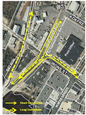
Figure 16: Short term recommendation for bicycle circulation is for Irons to be one-way bike lane out of downtown and for Herflicker and other back streets to link to Bus Depot via Highland Parkway. Long term connection to Bus Depot would be via rail R.O.W
