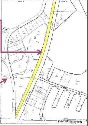
Figure 3: Tax Map from South Toms River showing Block 23, Lots 1 and 1.02 as potential right-of-way for future multipurpose path
