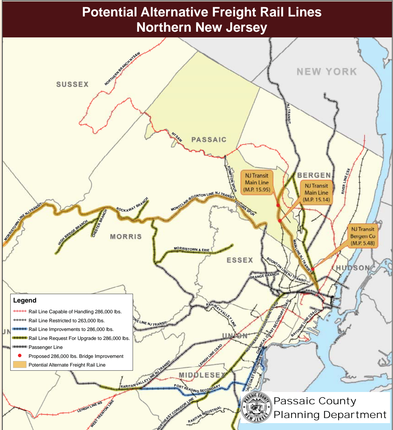
Figure 7.3 - Potential Alternative 286K Compatible Freight Rail Lines in the Northern New Jersey Area
