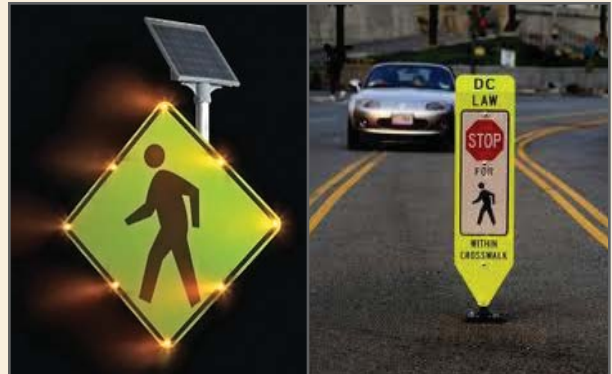
Installations such as blinking pedestrian signage and “stop for pedestrian” signage in the roadway can assist in making intersections and mid-block crossings safer.
