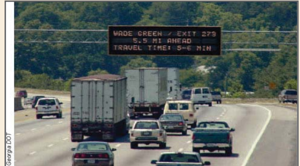
Variable Message Signs (VMS) and Dynamic Message Signs (DMS) can help inform drivers of prevailing conditions and plan alternative routes.
