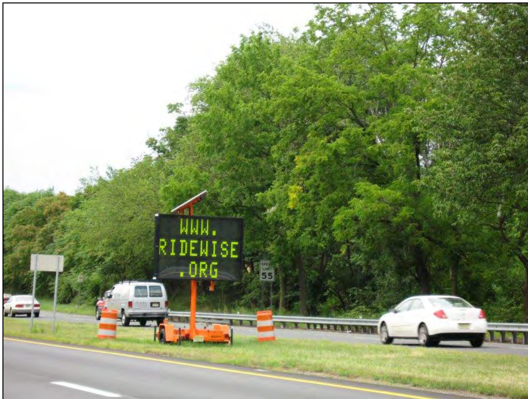
Figure 3-9 Variable Message Sign
