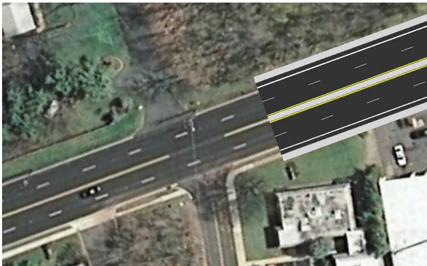
Cut away sketch of the configuration of Easton Avenue with a median barrier installed – a minimum of 3-5 feet of widening could be required on both sides of Easton Avenue.
