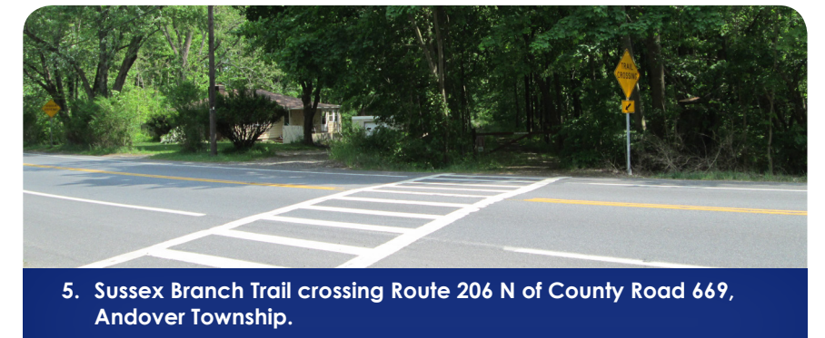
5. Sussex Branch Trail crossing Route 206 N of County Road 669, Andover Township. Trail crossing signs on roadway with a painted crosswalk where the trail crosses the roadway are present. This is one of three state highway crossings that were installed by NJDOT at the request of Sussex County. Others are pending as they are mid-block and require additional approvals.
