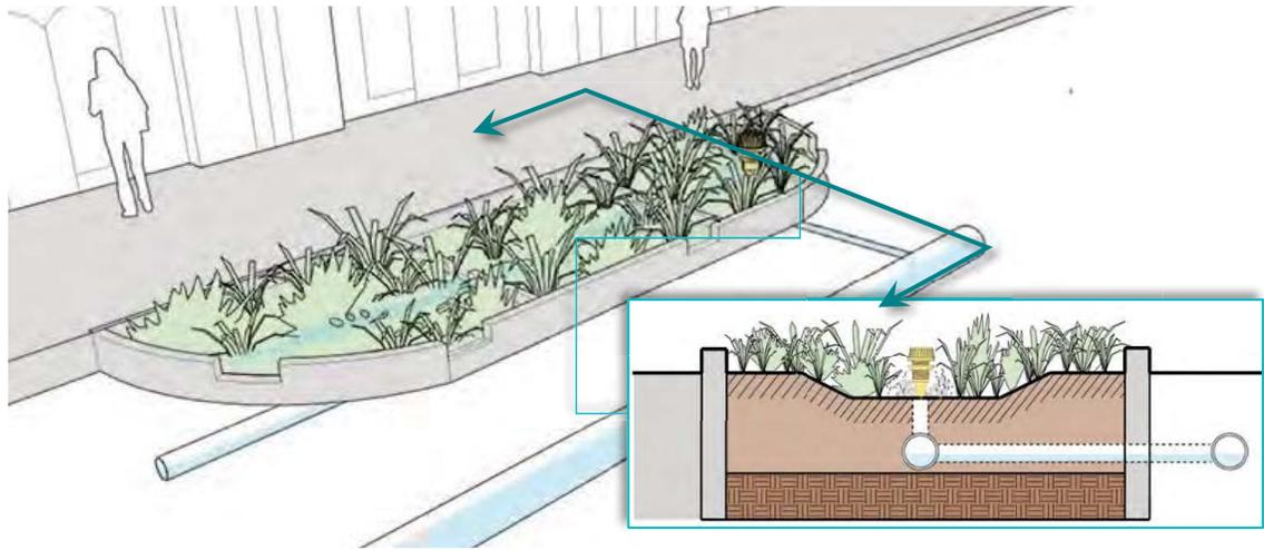
**Figure 16 – Example of Bioswale**
