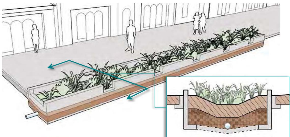
**Figure 17 – Example of Pervious Strips**
