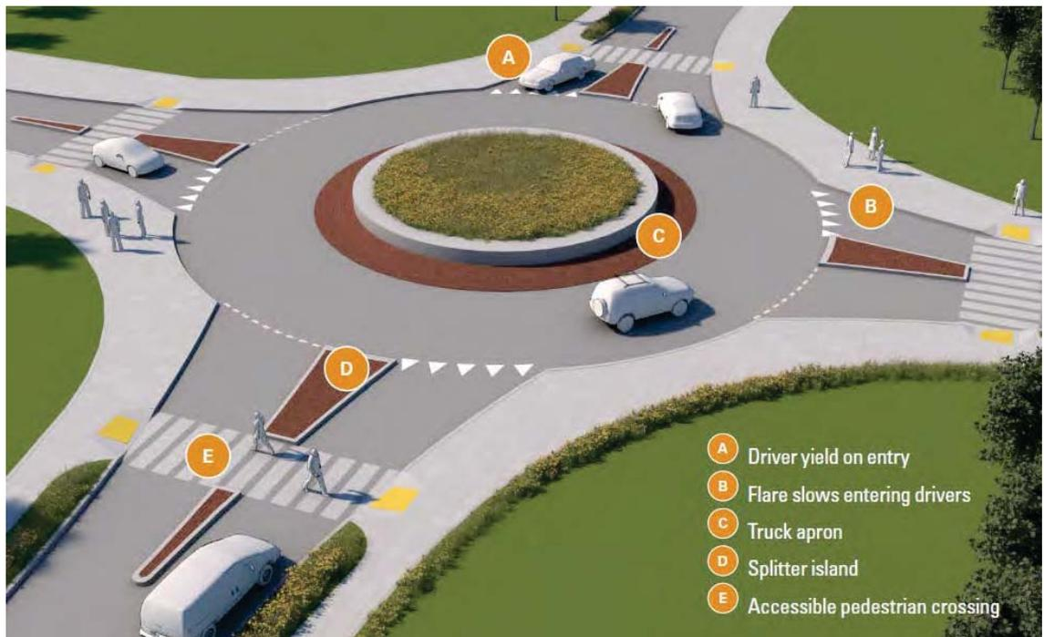
**Figure 15 – Roundabout Example (Source: CSDG)**
