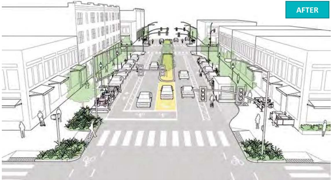
**Figure 14 – Typical Road Diet Application on a Main Street Typology (Source: NACTO-US)**
